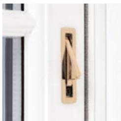
**Limit Stops** - Some windows may have limit stops fitted on the top sash. This opening restrictor allows for the top or bottom sash to be opened to a set position of 100mm. This needs to be pressed in or locked in position using the black nylon key provided to allow the sash to travel past it.
